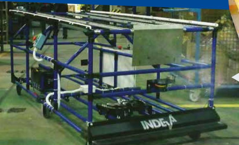
An INDEVA® custom gravity AGV is used to transport boxes and small containers in both directions between the warehouse and assembly line. The loading/unloading of the boxes from/to the AGV is carried out with a completely automatic and simple mechanism using gravity to slide boxes from the AGV to the rack and vice-versa. The dimensions of the roller tracks are designed according to the size and the number of boxes to be carried.
